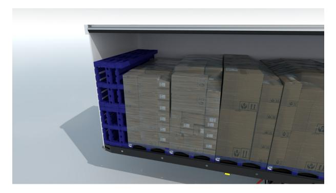
An example of blocking placed between the load and the headboard to prevent the load from moving forward.
