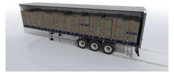
An example of a load secured correctly using lashing straps attached to the trailer chassis rave.
