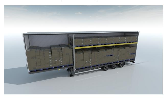
A fully loaded double deck XL rated trailer - the pallets on the upper deck weigh up to a maximum of 400kg and the heavier pallets are on the main and swan deck.
