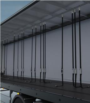
Left: example of black buckle straps hanging from the side of the vehicle roof.Right: example of black buckle straps hanging from a central track.
