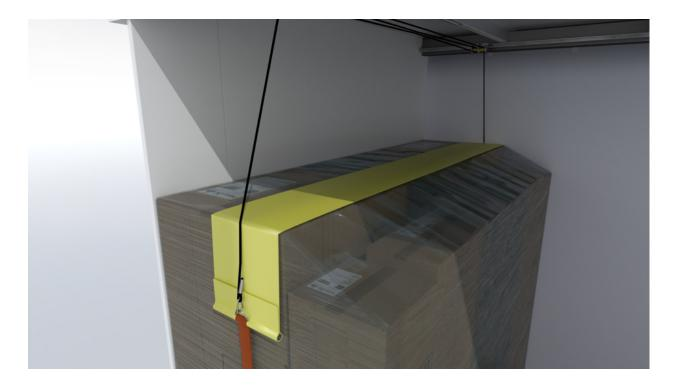
An example of a wider lashing strap, which distributes forces over the load. Although it's not being used on a bulk bag in this example, a wider lashing strap can help to spread the forces over bulk bags, as well as bales and boxes.
