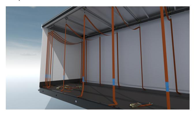
An example of normal lashing straps suspended by a bungee system.
