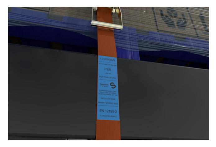
An example of a label attached to a lashing strap.
