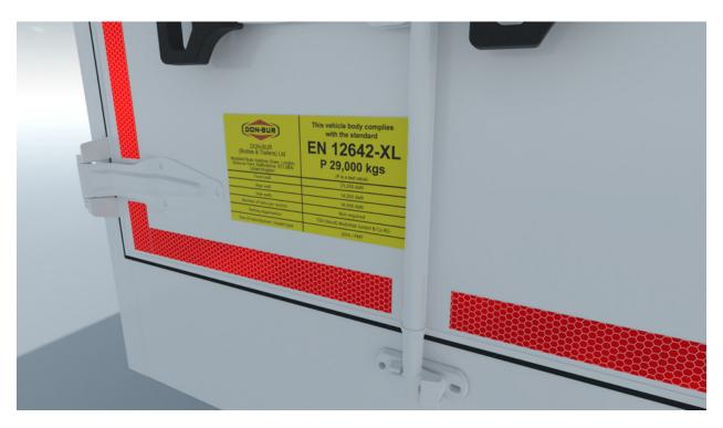
A vehicle built to BS EN 12642 standard will always display a label with build details.
