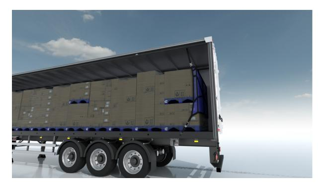
An example of a kite providing security at the rear of a load.
